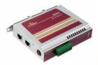
The SE5300 is a two or four serial ports to two Ethernet ports Industrial serial device server, which is an easy and reliable solution for bridging your serial based equipments to the Fast Ethernet networks. The two Ethernet ports can backup each other to provide redundant network connections for the serial devices connected to the SE5300. The serial ports support RS-232/422/485 or isolated RS-422/485, and the LAN ports support 10/100BASE-TX or 100BASE fibre optics.
